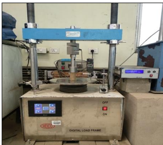
Fig. 5: Uniaxial compressive strength testing setup for rock and soil samples.
